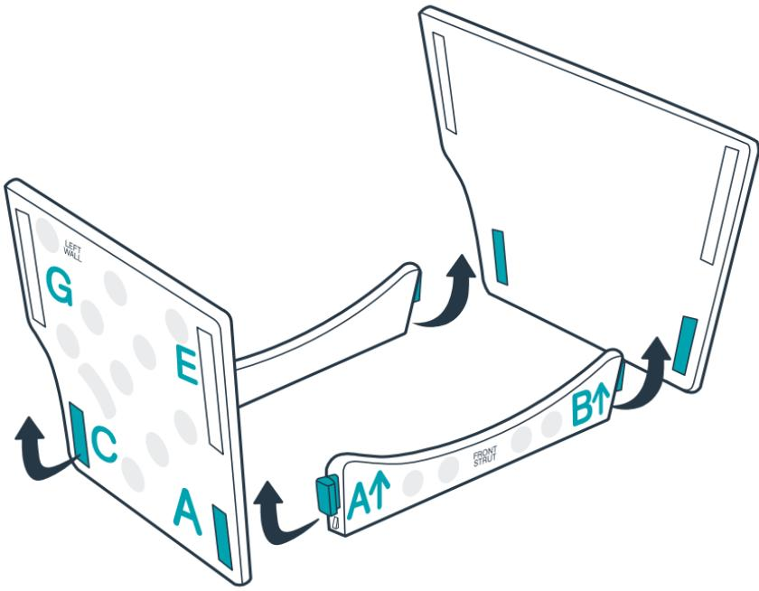
**EN** Attach the front and rear struts to the left and right walls of the safety seat frame, matching the letters on the tabs and slots. The smooth sides should face inwards. Press up on each strut to lock it in place.
